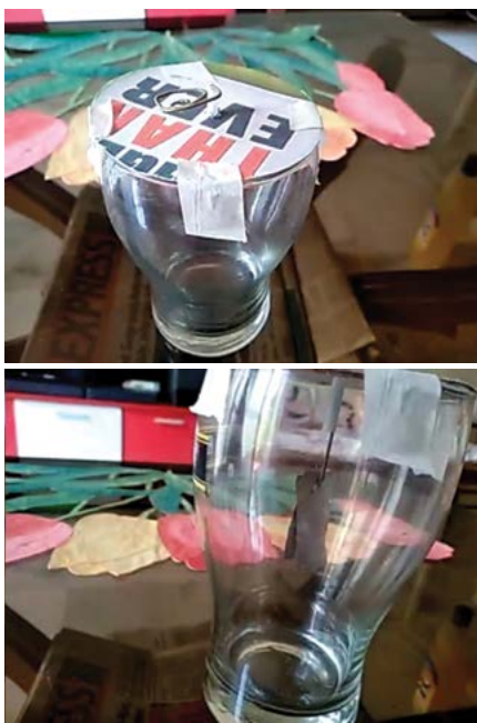
Fig. 1. Electroscope built by Divya. (a) A top-view, where the spiral shape of the copper wire is visible. (b) A side-view, in which the aluminium foil leaves are visible.
